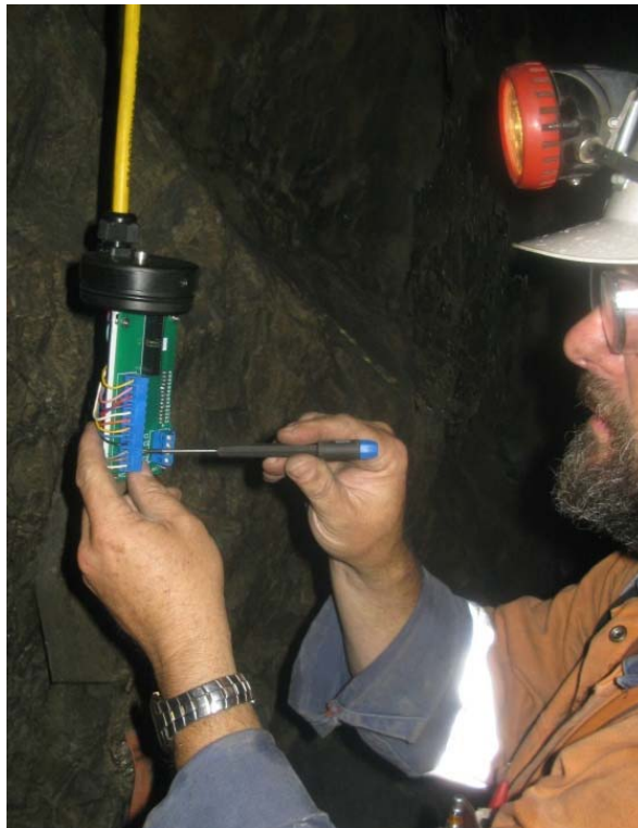
Connecting an HI Cell to an HIC termination end cap in the field
