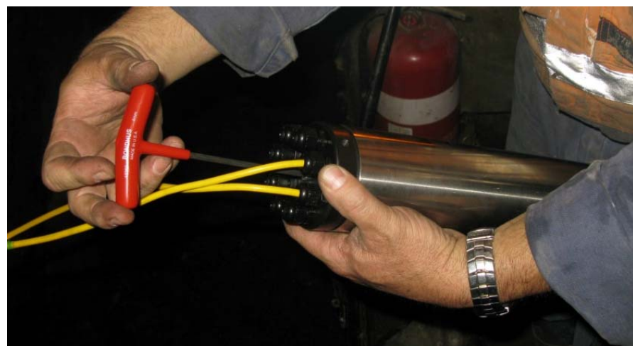
Completing reassembly of logger following connection of instruments
